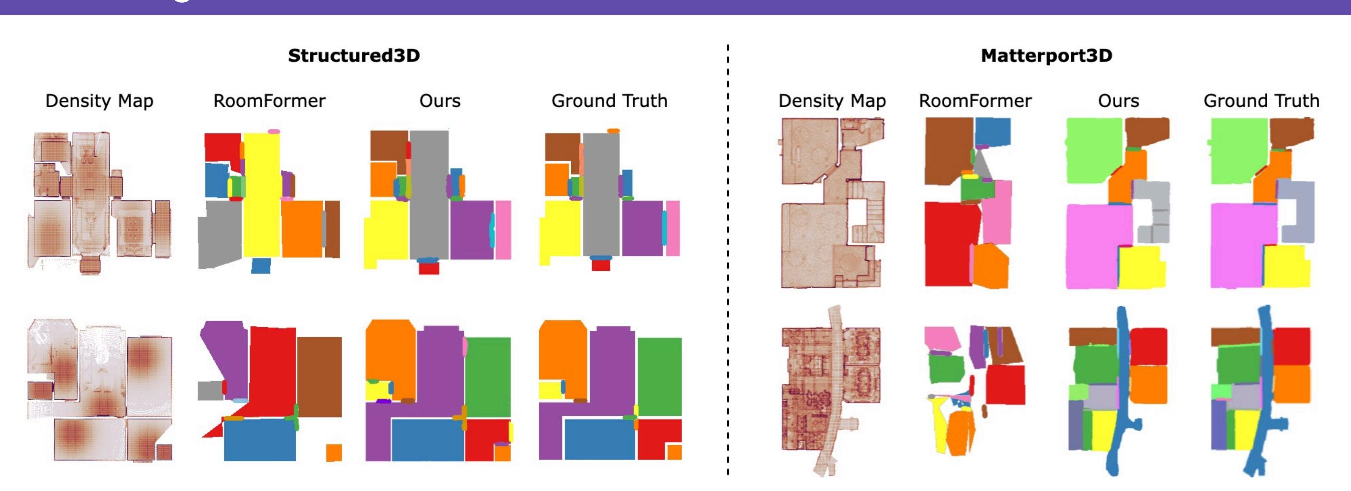
Our proposed method is able to handle adverse cases such as regions of low density (introduced by the scanning strategy) in the Stuctured3D dataset, as well as curved walls and clutter as seen in the Matterport3D dataset. Note: The colors only denote instance separation.
