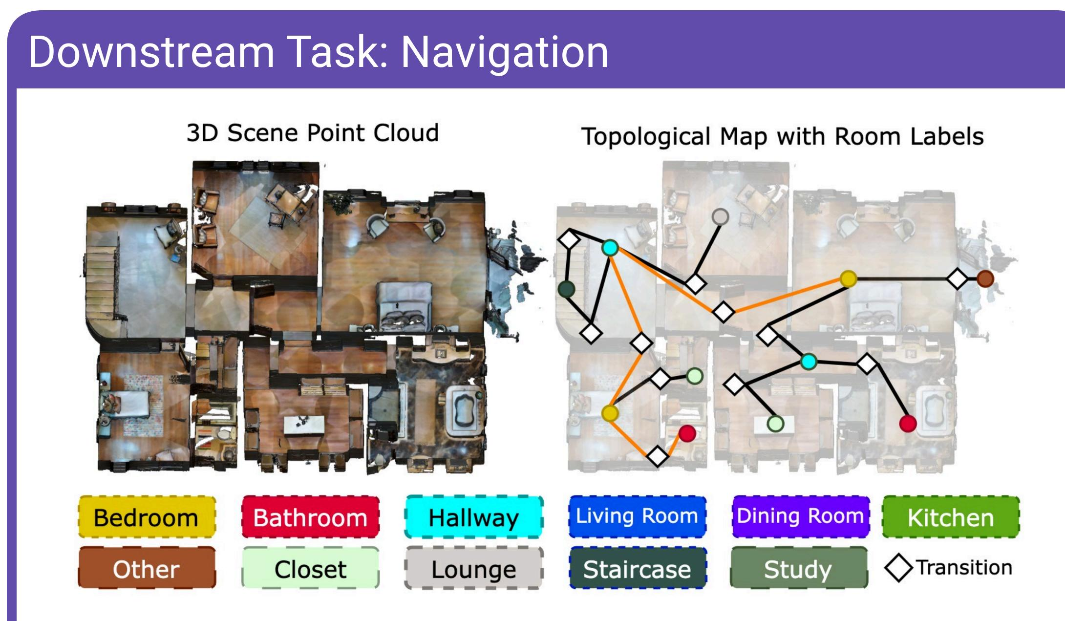
Detected transition regions aid in building a room-level topological map which can be used for tasks such as room-to-room navigation using natural language commands.
